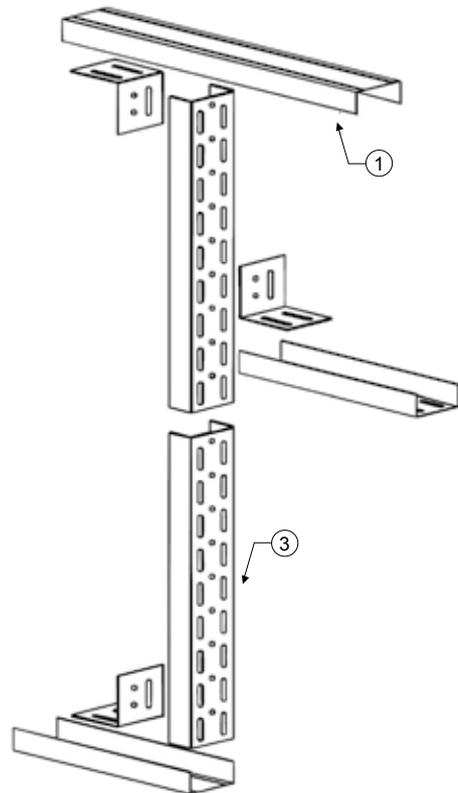
**TECHNICAL NOTES:** Secure to both the ceiling and the UA profiles on the floor with suitable fixings.
