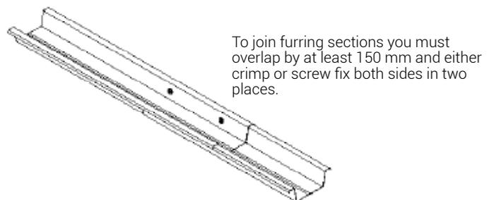
To join furring sections you must overlap by at least 150 mm and either crimp or screw fix both sides in two places.
