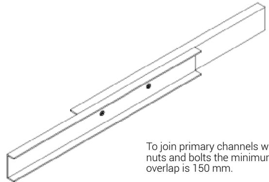
To join primary channels with nuts and bolts the minimum overlap is 150 mm.
