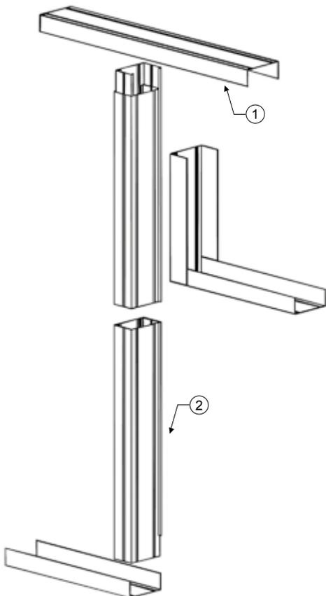
**TECHNICAL NOTES:** we suggest you insert a timber infill into the joined studs to create a wooden core.
